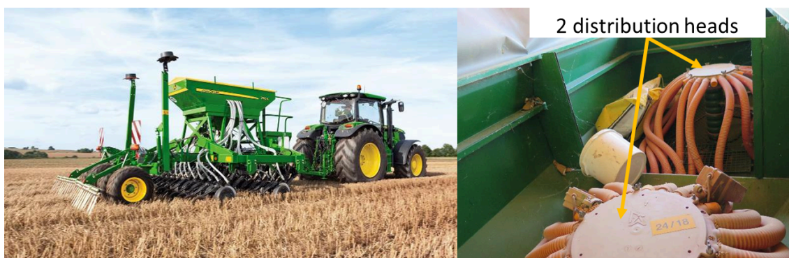
Figure 4: Illustration of a tinkered agro-equipment to sow two species simultaneously. Credit: E. Fouillet, INRAE.
