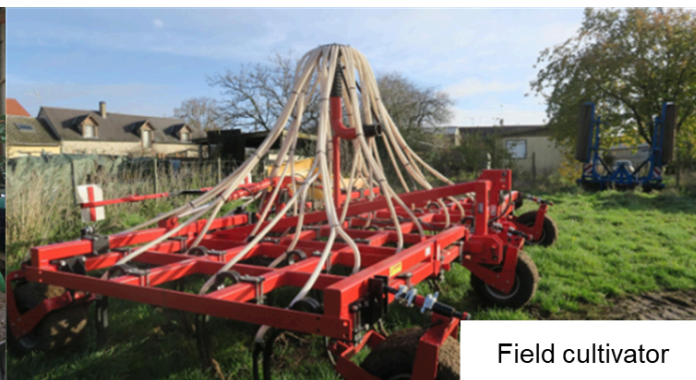
Figure 5: Illustration of a modified combined agricultural agro-equipment that can sow two species at different depths in a single pass. Credit: E. Fouillet, INRAE
