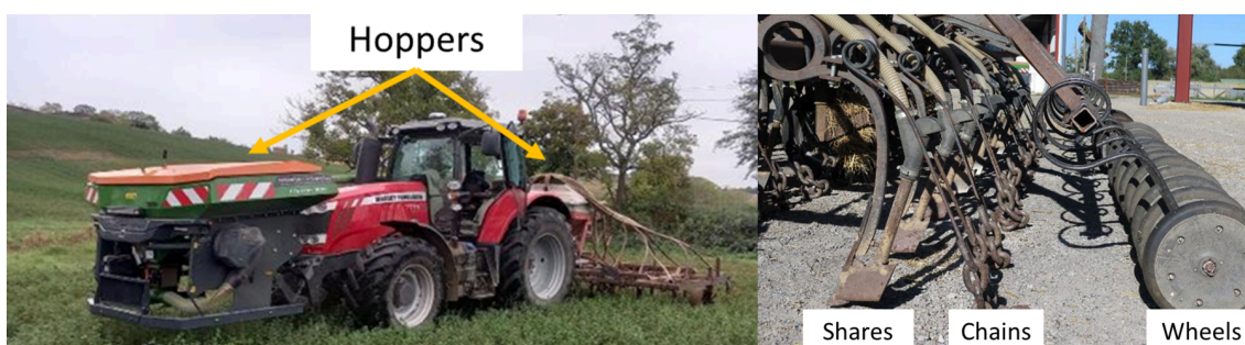
Figure 6: Illustration of the construction of a no-till drill to sow several species simultaneously. Credit: E. Fouillet, INRAE
