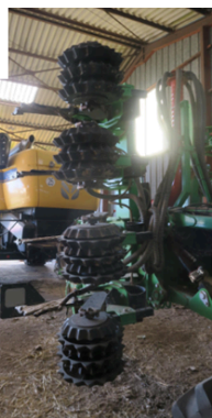
Figure 5: Illustration of a modified combined agricultural agro-equipment that can sow two species at different depths in a single pass. Credit: E. Fouillet, INRAE
