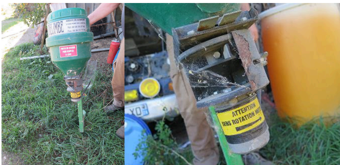
Figure 3: Illustration of a repurposed agro-equipment, namely that of a micro granulator electric distribution initially designed for spreading fertilizer and repurposed here for sowing cover crops. Credit: E. Fouillet, INRAE.
