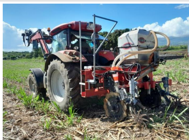
Figure 2: Disc seeder with straw cutter (for use with mulch). Photo: eRcane.
