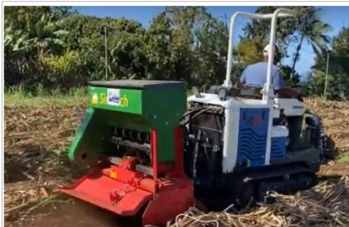
Figure 1: Micro-tractor seed drill (with mulch concentrated on the row). Photo: eRcane.
