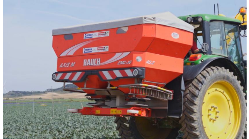
Figure 2: Sowing with centrifugal fertilizer spreader before last cultivation between lines. Photo: Telmo Fernández Ibarburu.
