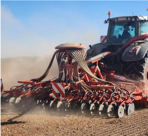
Figure 1: Sowing with mechanical seed drill before planting. Photo: Miguel Ángel Los Arcos, farmer of Santiago Apóstol Cooperative.
